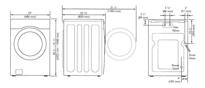
ASKO XXL washing machines are shipped with a cord for connection to a 120 V, 15 Amp single phase electrical circuit. There are two fill hoses for connection to the hot and cold water supply. The XXL washing machine has the capability of draining upwards 8' (244 cm).
